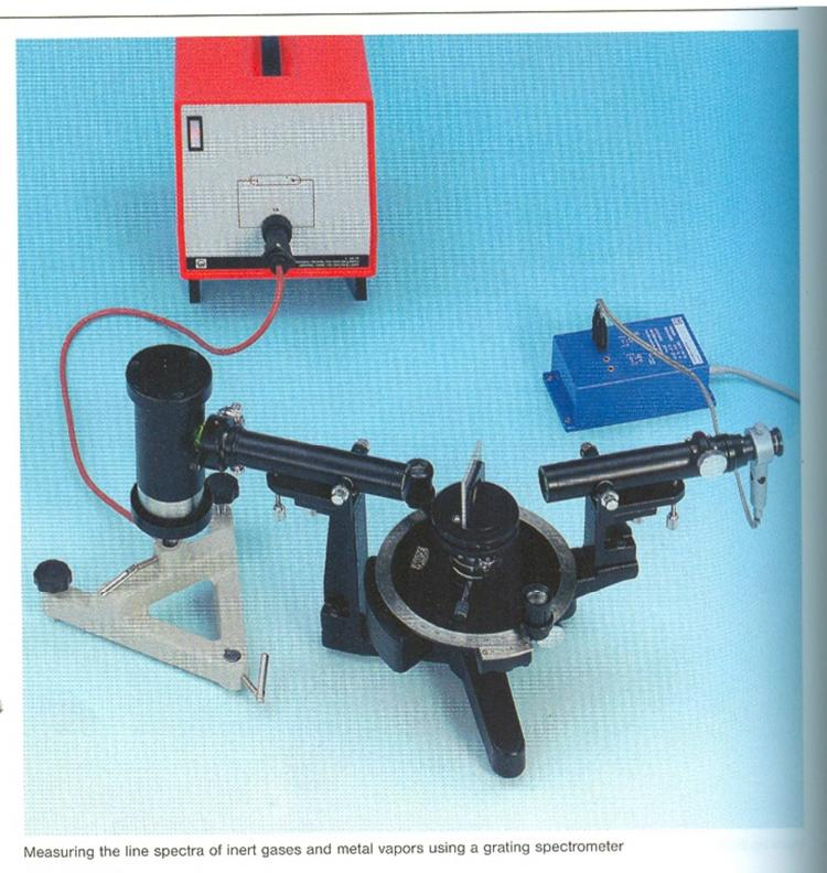
Measuring the line spectra of inert gases and metal vapors using a grating spectrometer
